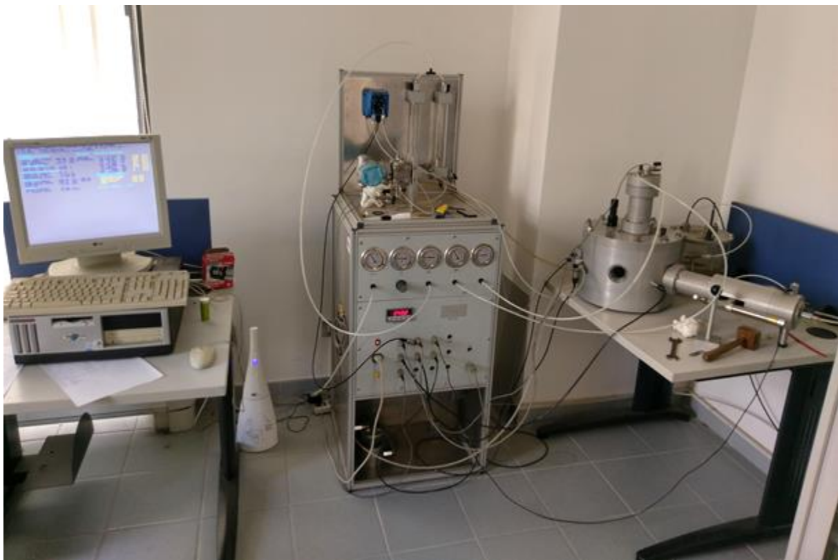
Figure 74: Suction Controlled Direct Shear Apparatus (SCDSA) (Megaris s.a.s.) used in the Geotechnical laboratory at the UniSa.
