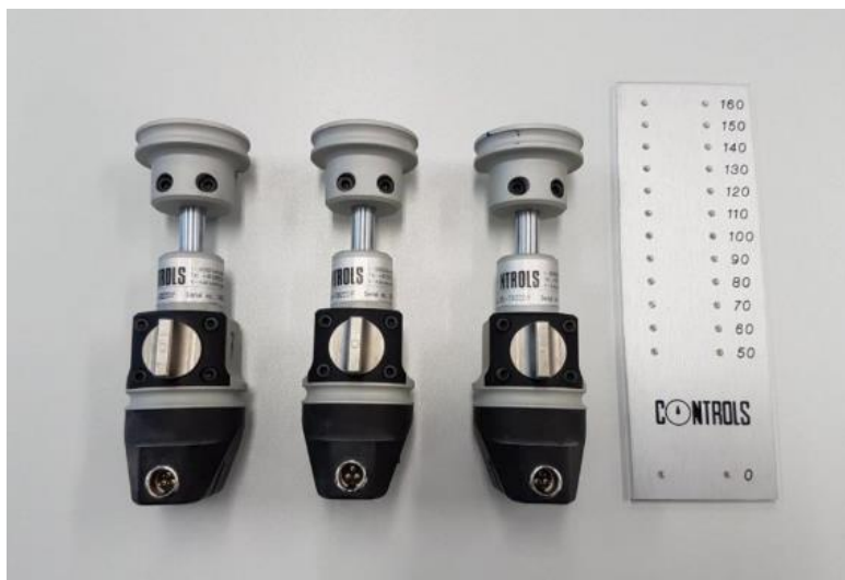
Slika 36: LVDT uređaji (linear variable differential transformer)
