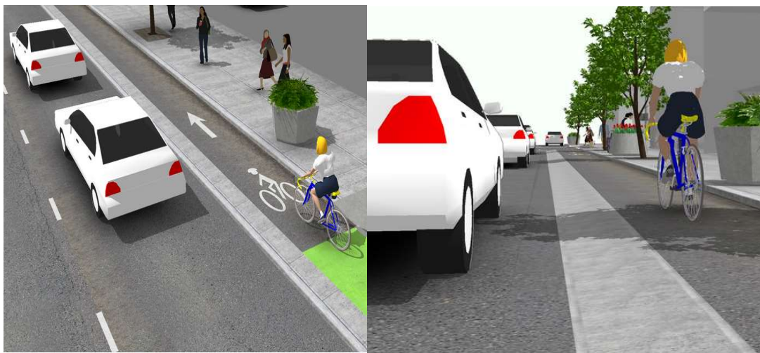
Figure 45: Examples of an elevated protected cyclist lane [12]
